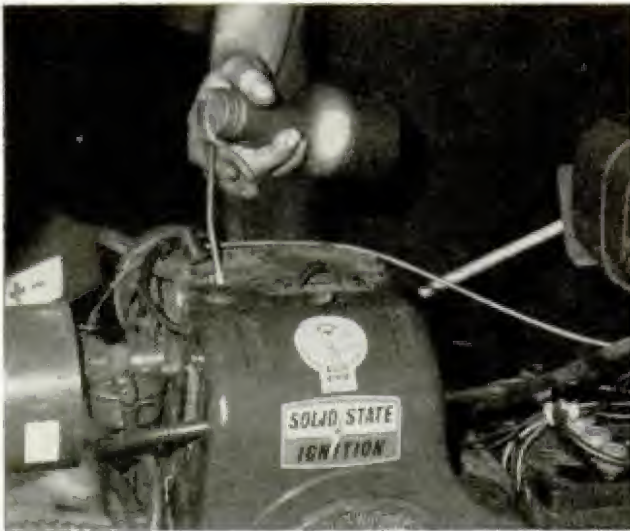
FUEL REACHING CYLINDER? Squirt some in plug hole, replace plug. If engine starts, then stops when this has burned, fuel line or screens are blocked
